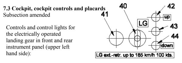
40) Toggle switch for extension and retraction of the electrically operated main landing gear
