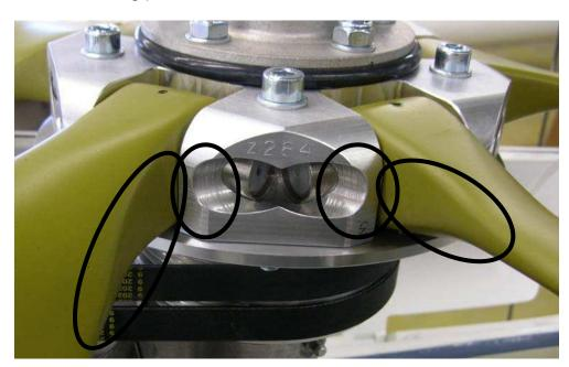
Check propeller blades for ease of movement. Each blade should unfold automatically when it is in the bottom position, otherwise the bearing at the blade root should be lubricated with thin oil.
